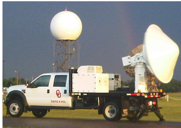
Figure 1. RaXPoI radar deployed in a severe thunderstorm on 14 June 2011 in central Oklahoma (photo by A. Pazmany).
